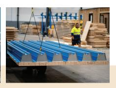
Strongfloor is a Timber Concrete Composite developed and tested by Viridi Group, utilising timber where it performs best. Timber acts in tension at the base of the floor, provides a high quality aesthetic soffit, and acts as permanent formwork to the concrete. Steel channels are fixed in a factory setting in composite action to the mass timber panels providing strength, while concrete is poured over the top to provide a robust and solid finish under foot.
